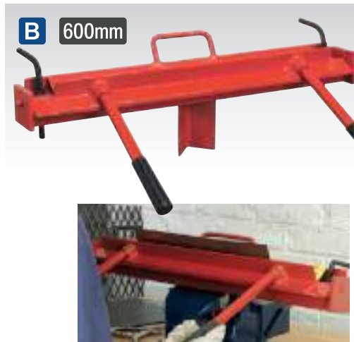
B DF600 600mm Vice Mounting Metal Folder Suitable for use in a sturdy bench mounted vice and capable of bending up to 22 gauge steel sheet. Ideal for small garage or restoration operation. Capacity: 600mm x 22 Gauge Sheet, Ø2mm Rod
