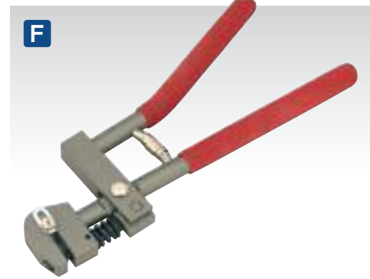
F RE92/35 Ø5mm Punch Tool All steel construction with spring loaded handles. Ø5mm Holes are suitable for preparing panels for MIG/spot welding. Fitted with non-slip PVC grips.
