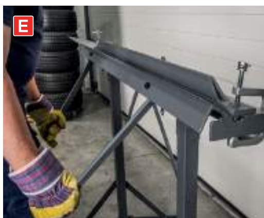
D TS01 700mm Vice/Bench Mounting Sheet Metal Folder Bench and vice mounting sheet metal folder, fitted with mounting plates. Capable of bending up to and beyond a 90° angle. The unique patented 'endless' design and removable folding plate allows the user to fold, channel and offset any length of sheet metal up to 20 Gauge/0.91mm thick. Capable of two folds at right angles to each other to form a corner piece. With adjustable fold plate to help achieve the cleanest fold possible. Ideal for the small garage or restoration operation. Capacity: 700mm x 20 Gauge Sheet, Ø1mm Rod
