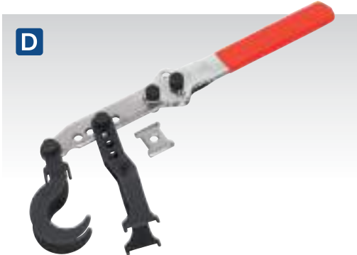
D VS168 OHV Valve Spring Compressor Suitable for the replacement of valve springs and valve stem oil seals without the need to remove the cylinder head. Use in conjunction with Model No. VS1601 compressed air adaptor. Adjustable handle, claws and hooks allow use on most OHV engines. Note: Not suitable for vehicles with deep-seated valves.
