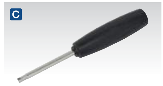
C TST18 Torque Limited Tyre Valve Tool Pocket size tool specifically designed to prevent over tightening of valve cores fitted to wheels/tyres with TPMS. Over-torquing can easily damage delicate pressure sensor packs, causing expensive repairs. Preset Torque: 0.48Nm (4lb.in)
