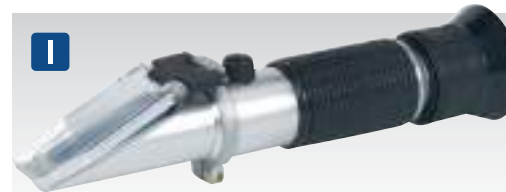
I VS005 Refractometer Antifreeze/Battery Fluid/Screenwash Accurately measures the strength of battery fluid, screenwash and antifreeze by measuring the refractive index of light passing through the mixture. Suitable for synthetic antifreeze mixtures including long life OAT (Organic Acid Technology) and G13. Temperature corrected prism ensures accuracy. Eyepiece with adjustable focus. Supplied with pipette and storage case.
