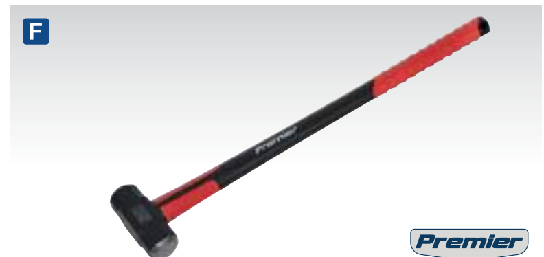
F SEE BELOW Sledge Hammers with Fibreglass Shaft Manufactured from fine grained carbon steel. Heat treated, induction-hardened and tempered with precision ground polished striking face. Fitted with fibreglass shaft and contoured shock-absorbing rubber grip. Manufactured in accordance with BS 876.
