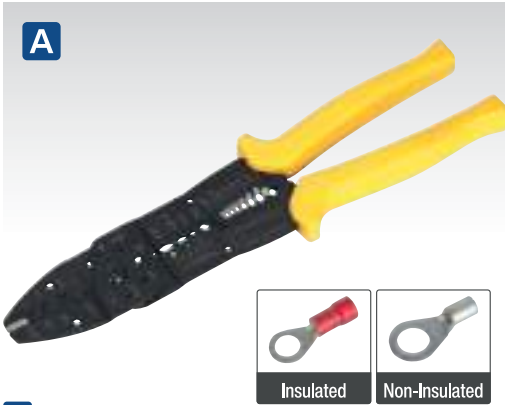
A AK3851 Stripping & Crimping Tool 3mm Steel construction with safety insulated handgrips. Crimps insulated terminals 0.5-6mm 2 . Crimps non-insulated terminals 1.5-6mm 2 . Crops threaded terminals M2.6-M5. Strips wires 0.75-6mm 2 . Also fitted with wire cutters for soft cables and wires. Length: 250mm
