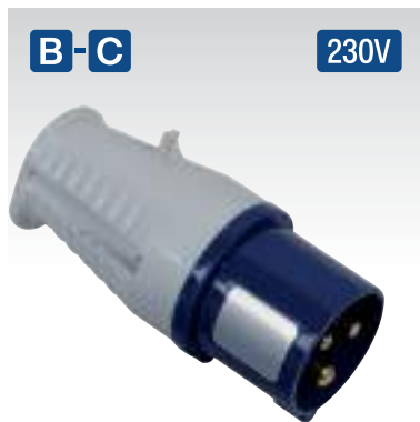
B-C SEE BELOW 230V 2P+E Blue Plugs 230V Plugs, IP44 rated, 16A. 2P+E Connector. Conforms to BS EN 60309. B Model No: WP24016 Description: 16A/230V C Model No: WP24032 Description: 32A/230V
