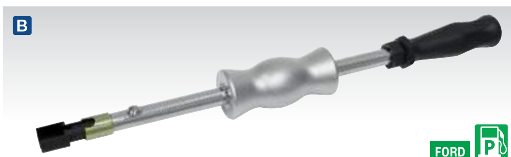
B VS2067 Petrol Injector Puller - Ford EcoBoost Extracts petrol injectors easily without damaging the injector or head. Includes slide hammer and specially designed injector claw. Equivalent to OEM 310-206. Applications: Ford; GDi & GTDi EcoBoost engine ranges from 1.0L to 2.3L
