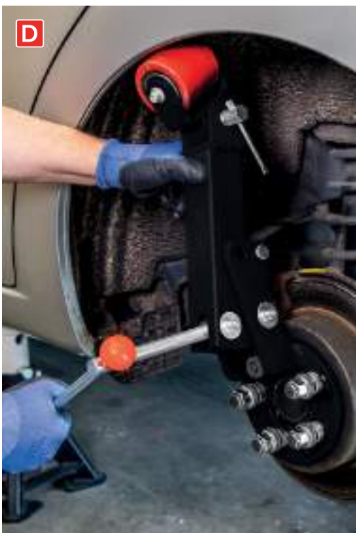
D SAR01 Wheel Arch Reshaping Tool Reshaping tool designed for repairing wheel arch collision damage or for increasing tyre-to-wing clearance by flaring wheel arches. Fully adjustable telescopic arm that allows 180° wheel swivel. Elongated holes on the hub adaptor plate suitable for vehicles with various four and five stud/bolt patterns. Bolts directly to the hub assembly. Attached hitch pin allows for change in angle. Min./Max. Arm Length: 440/560mm
