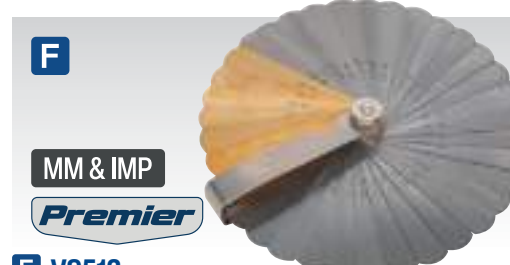
F VS513 36 Blade Combination Steel/Brass Feeler Gauge - Dual Marked 30 Steel blades and six brass blades for non-magnetic applications on electronic ignition systems. Blade dimensions 75 x 13mm. Blade Sizes: Imperial Steel: 0.002", 0.0025", 0.003", 0.004", 0.005", 0.006", 0.007", 0.008", 0.009", 0.010", 0.011", 0.012", 0.013", 0.014", 0.015", 0.016", 0.017", 0.018", 0.019", 0.020", 0.021", 0.022", 0.023", 0.024", 0.025", 0.026", 0.028", 0.030", 0.032", 0.035" Imperial Brass: 0.006", 0.008", 0.010", 0.012", 0.014", 0.016" Metric Steel: 0.051, 0.063, 0.076, 0.102, 0.127, 0.152, 0.178, 0.203, 0.229, 0.254, 0.279, 0.305, 0.330, 0.356, 0.381, 0.406, 0.432, 0.457, 0.483, 0.508, 0.533, 0.559, 0.584, 0.610, 0.635, 0.660, 0.711, 0.762, 0.813, 0.889mm Metric Brass: 0.152, 0.203, 0.254, 0.305, 0.356, 0.406mm
