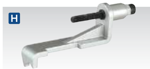
H VS151 Rocker Arm & Valve Compensator Tool Suitable for use on Vauxhall/Opel OHC engines. Permits quick, on-vehicle, removal of rocker arm and valve play compensator. Mounts on camshaft housing. Cast construction with knurled hex head fixing.
