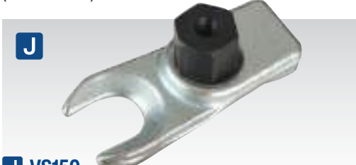
J VS150 CVH Valve Spring Compressor - Ford Permits valve stem seal and valve spring replacement without the need to remove the cylinder head. Superior cast design with radiused fulcrum for smooth spring compression. Suitable for CVH Ford engines 1.3, 1.4 and 1.6 as fitted to Escort (inc. XR3i and RS Turbo) and Fiesta (inc. RS Turbo).
