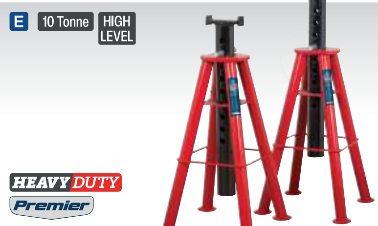
E AS10H High Level Axle Stands (Pair) 10 Tonne Capacity per Stand Heavy-duty high level axle stands to safely support vehicles for extended periods of time. Large crutch for even load distribution. Heavy gauge steel frame and welded construction give superior strength and safety. Features captive, multi-position pin load support. Ideal for commercial vehicles. Sold in pairs.
