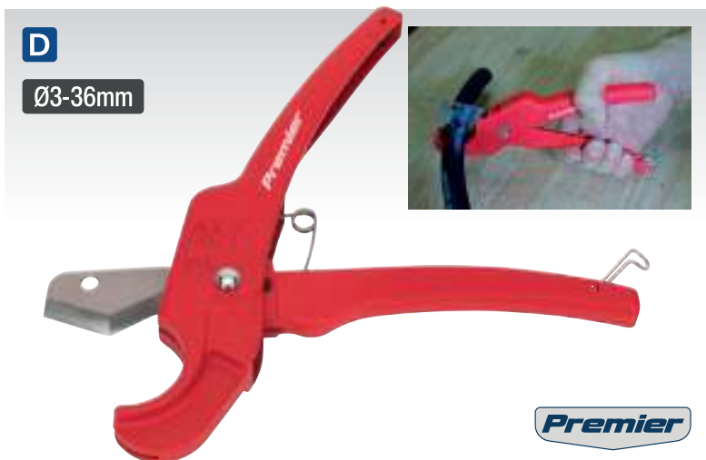
D HCA26 Rubber & Reinforced Hose Cutter Powder coated aluminium body. Operates with a simple plier action. Heat treated stainless steel cutting blade. Locking mechanism for safe storage. Suitable for hoses from Ø3-36mm. Capacity: Ø3-36mm Length: 220mm
