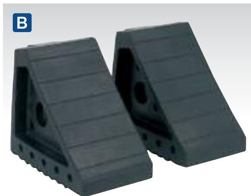
B WC01 Rubber Wheel Chocks 1.8kg - Pair Two rubber wheel chocks. Prevents vehicle movement when being jacked on a level surface or parked on an incline not exceeding 12°. Suitable for vehicles below 3 Tonne. Dimensions (W x D x H): 100 x 195 x 150mm
