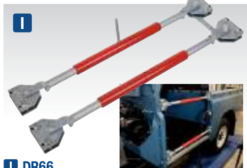
I DR66 Door Restraining Bars - Pack of 2 Manufactured with steel tube and heavy jaw assemblies. Designed to triangulate and strengthen door apertures whilst performing pulling operations. Supplied with tommy bar. Minimum Length: 830mm Maximum Length: 1160mm Jaw Width: 90mm
