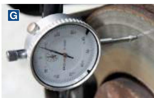
G VS0290 Brake Disc Run-Out Kit Check for ball joint wear and brake disc run-out quickly and easily. Locking pliers secure to any convenient position, enabling DTI gauge to be placed against brake disc. Kit includes Metric calibrated DTI gauge. Deflection/Travel: 10mm Graduation: 0.01mm Shank Size: 8mm
