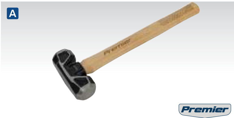
A SLH041 4lb Short Handle Sledge Hammer with Hickory Shaft Manufactured from drop-forged fine grained carbon steel. Heat treated, hardened and tempered with precision ground polished striking face. Straight-grain hickory handle. Manufactured and tested to BS 876.
