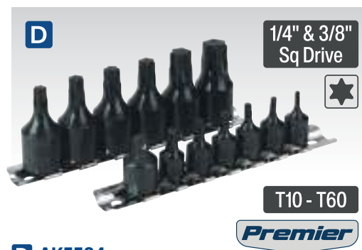
D AK5584 13pc 1/4" & 3/8" Sq Drive TRX-Star* Socket Bit Set Drop-forged one-piece Chrome Vanadium steel, specially hardened and tempered. Finished in black oxide for corrosion resistance. Supplied on two rails. Drive: 1/4" & 3/8" Sq Contents: 1/4" Sq Drive; T10, T15, T20, T25, T27, T30, 3/8" Sq Drive; T40, T45, T47, T50, T55, T60, 3/8" Sq(F) x 1/4" Sq(M) Adaptor Minimum/Maximum Length: 25/40mm
