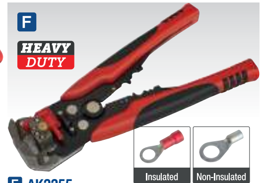
F AK2255 Heavy-Duty Automatic Wire Stripping Tool Heavy-duty, professional automatic wire stripper with alloy steel jaws. Fully automatic, single action, grips and strips all types of wire 0.2-6mm 2 with minimal pressure to handles and no damage to the inner core of the wire. Adjustable length stop is easily swivelled to allow longer stripping. Precision machined wire cutting blades for long-life. Features three crimping elements for insulated, non-insulated (1.5-6mm 2 ) and auto-ignition terminals (7-8mm). Stripping Capacity: 0.2-6mm 2 Length: 200mm
