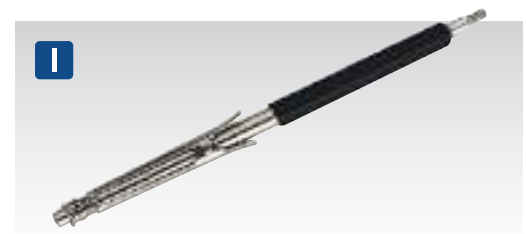
I VS1651 Valve Collet Installer/Remover 8/16/24 Valve Spring loaded shaft and clips aid simple and secure installation of valve spring collets. Quick and easy retrieval of lost collets using magnetic tip. Suitable for 8, 16 and 24 valve engines. Ideal for use on heads with recessed valves.
