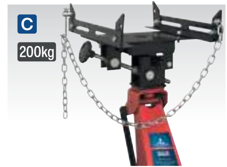
C ADT200 200kg Capacity Transmission Cradle Fully adjustable saddle with forward, backward and side-to-side tilt. Suitable for jacks with a 31-33mm saddle spigot pin.
