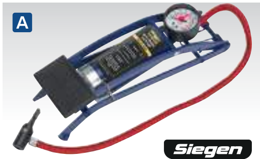
A S0540 Single Barrel Foot Pump Steel framed foot pump with Ø50 x 120mm steel barrel. Dial type pressure gauge with rotating bezel. Gauge calibrated in psi and bar and ranges from 0-100psi and 0-7bar. Fitted with 610mm of flexible pressure hose with clip-on type connector. Supplied with accessory for inflating items such as small inflatable boats, air beds and balls.
