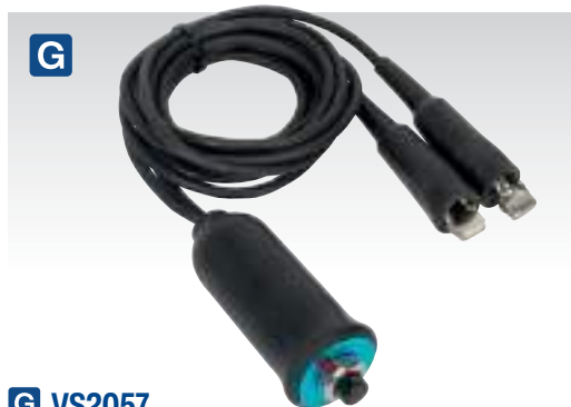
G VS2057 Remote Starter Switch One-person operation, suitable for turning the engine over for various diagnostic tasks such as compression testing. Connects to the starter system with push-button activation. Features a connectivity LED and 1.5m cable.
