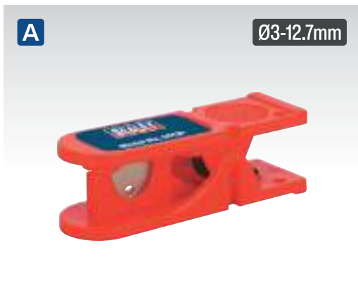
A SC127 Rubber Hose Cutter ABS body with steel, heat treated blade to hardness of 50-55 HRC. Capacity: Ø3-12.7mm Length: 80mm
