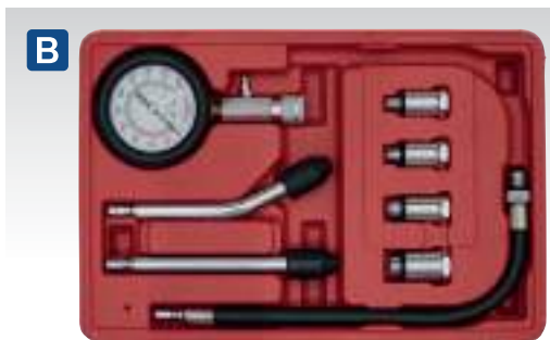
B CT955 8pc Compression Test Kit Compression tester fitted with Ø63mm gauge reading up to 300psi(20kg/cm 2 ). Kit includes 130mm straight and angled push-on connectors, 300mm flexible extension with 10, 12, 14, 18mm adaptors.
