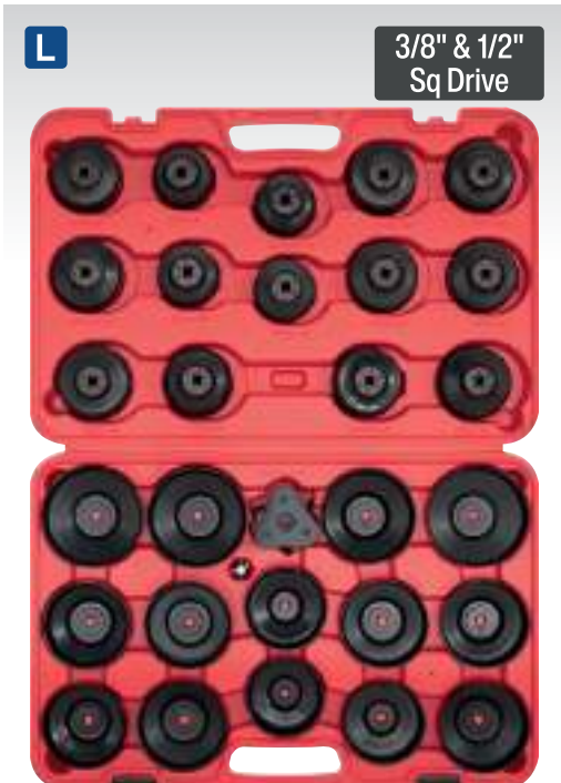
L VS7006 30pc Oil Filter Cap Wrench Set Extensive set designed for a wide range of vehicles. Cap type filter wrenches, made from 7 and 16 gauge steel, will withstand up to 115Nm(85lb.ft) of torque. Designed to grip like sockets, thereby minimising the possibility of crushed filters. Includes adjustable oil filter wrench. Adaptor allows use with 3/8" or 1/2" Sq drive wrenches.
