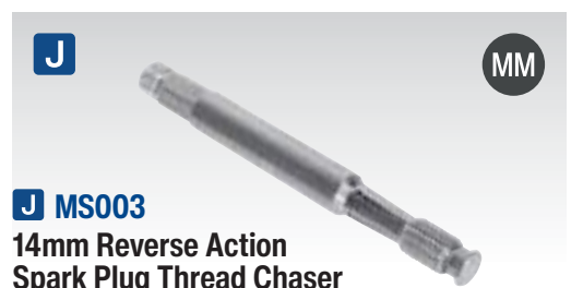
J MS003 14mm Reverse Action Spark Plug Thread Chaser Specially designed to repair damaged spark plug threads on modern engines. Unique design allows the tool to be passed through the plug thread into the combustion chamber, then expanded to the correct size starting on the inner, undamaged threads. Traditional thread restorers rely on luck for the restored and undamaged threads to align. Size: 14mm Length: 138mm
