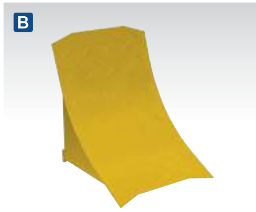
B WC17 Heavy-Duty Steel Wheel Chock - Single Welded steel wheel chock. Prevents vehicle movement when being jacked on a level surface or parked on an incline not exceeding 10°. Suitable for heavy goods vehicles not exceeding 15 Tonne gross weight.
