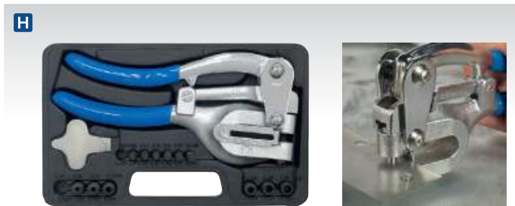
H AK9821 14pc Metal Punch Set Heavy-duty drop-forged and heat treated steel punch body with compound lever action. Suitable for precision punching of holes in steel, aluminium, brass, copper and plastic. Fitted with gauge for depth adjustment up to 50mm. Suitable for materials up to 14 gauge. Punches and dies hardened to 55-60 HRC. Supplied in storage case.
