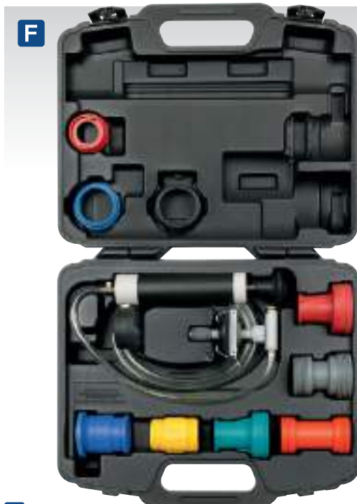
F VS0031 Cooling System & Cap Testing Kit Capless cooling system tester uses an inflatable bladder to seal the pressure head to the radiator or header tank. Bladder system can be used on both screw and bayonet fittings and seals 90% of cars and light commercial vehicles straight out of the box. Also suitable for motorcycles, off-road and marine applications. Supplied with a set of double end adaptors enabling testing of cooling system pressure caps. Supplied in storage case. Applications: Pressure Cap Test; Standard Bayonet (Ford, GM N Body), External Thread (Jeep, Saab, VW/Audi), Internal Thread (Small Japanese Deep, VW/Audi), Internal Thread (Small Japanese Shallow, Late Model VW/Audi), External Thread (Late Model BMW, Land Rover), External Thread (Late Model Mercedes), Pressure System; Universal
