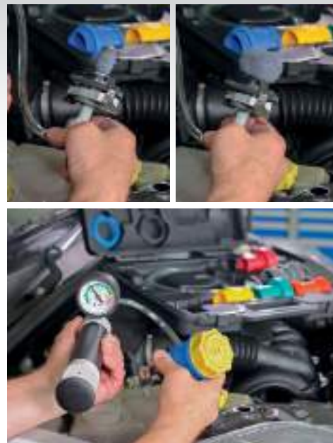
Kit includes cap test adaptors - simply insert bladder into adaptor and inflate.
