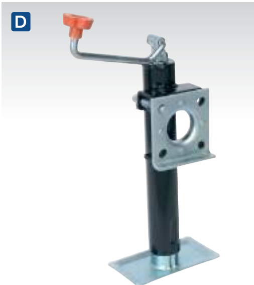
D TB373 Trailer Jack & Clamp 250mm Travel 900kg Capacity Heavy-duty trailer jack with swivel mounting. Suitable for handling trailers with heavy nose weight. Integral swivel weld-on mounting.
