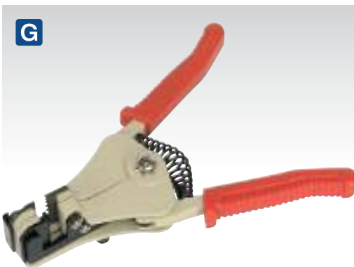
G AK2252 Automatic Wire Stripping Tool One-handed, compound action grips and strips electric cables 1-3.2mm 2 automatically. Jaw action prevents crushing or cutting even the finest wires. Supplied with length gauge and fitted with vinyl grips. Stripping Capacity: 1, 1.6, 2, 2.6, 3.2mm 2 Length: 175mm
