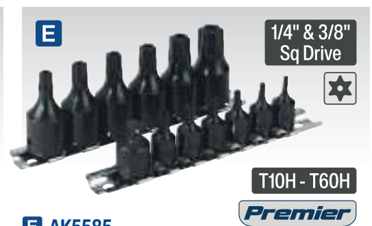
E AK5585 13pc 1/4" & 3/8" Sq Drive TRX-Star* Security Socket Bit Set Drop-forged one-piece Chrome Vanadium steel, specially hardened and tempered. Security TRX-Star* type head. Finished in black oxide for corrosion resistance. Supplied on two rails. Drive: 1/4" & 3/8" Sq Contents: 1/4" Sq Drive; T10H, T15H, T20H, T25H, T27H, T30H, 3/8" Sq Drive; T40H, T45H, T47H, T50H, T55H, T60H, 3/8" Sq(F) x 1/4" Sq(M) Adaptor Minimum/Maximum Length: 25/40mm
