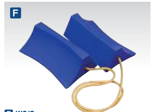
F WC15 Plastic Wheel Chocks - Pair Sturdy yet lightweight wheel chocks weigh around 250g each. Prevents car, caravan, or light aircraft moving when jacking or parked on an incline. Supplied on 800mm sturdy rope for easy storage and removal from underneath wheels. Not intended for use on sloped ground over 10°.
