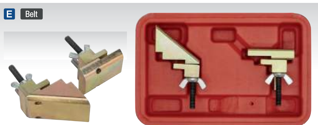
E VS787 Auxiliary Stretch Belt Removal/Installation Tool Designed for the recommended removal and installation of elasticated or stretch drive belts fitted to modern auxiliary drive systems, such as the alternator or power steering. Prevents damage to the pulley and prolongs the life of the belt. Two tools included, one for installation and one for removal. Fits most crankshaft pulleys. Supplied in storage case.
