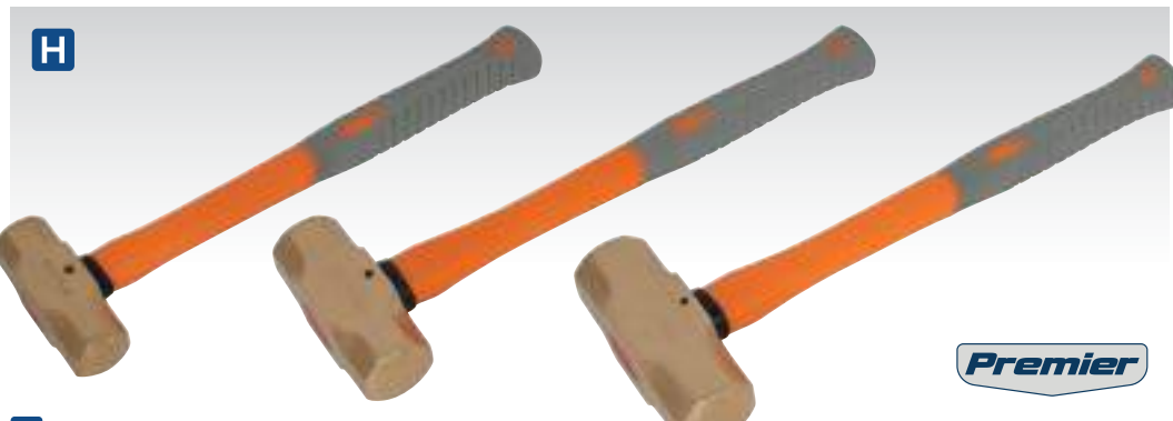
H SEE BELOW Sledge Hammers - Non-Sparking Precision cast Beryllium Copper heads. Fitted with fibreglass shaft and shock-absorbing grip for greater comfort and control. Manufactured in accordance with BS 876.
