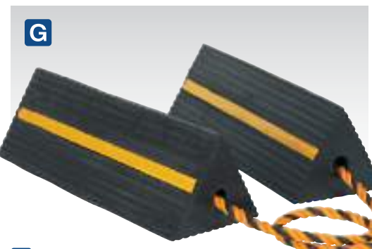
G WC11 Heavy-Duty Rubber Wheel Chocks 8kg - Pair Rubber wheel chocks weighing 8kg (4kg each) prevent vehicle movement when jacking or parking on an incline. Suitable for heavy commercial vehicles and light aircraft. Chocks supplied on rope for easy storage and removal from underneath wheels. Not intended for use on sloped ground over 12°.
