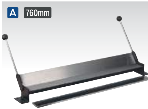
A DF760 760mm Bench Mounting Metal Folder Bench mounting sheet metal folder, fitted with mounting plates. Capable of bending up to 17 gauge steel sheet. Ideal for the small garage or restoration operation. Suitable clamps (not included) are required to secure the pressing plate for operation. Capacity: 760mm x 17 Gauge Sheet, Ø2mm Rod
