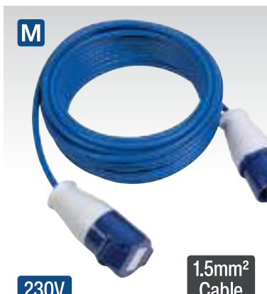
M EL1523016 14m Extension Lead 230V 16A 1.5mm 2 Extension cable fitted with 2P+E plug and socket connectors rated at 230V 16A with protective end cover. H05VV-F 3G 1.5mm Section cable. IP44 Rated. Length: 14m Cable Section: 1.5mm 2 Plug Type: Blue - 16A-2P+E
