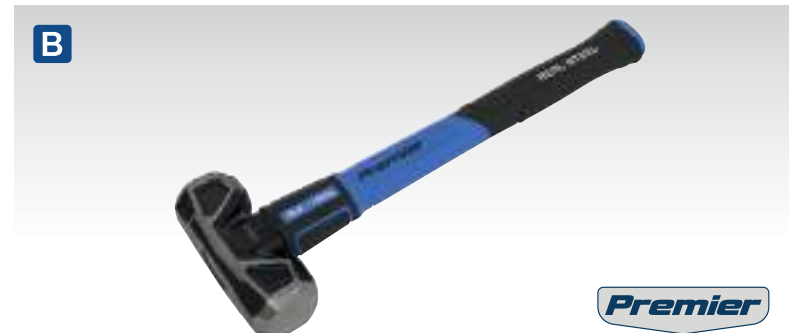
B SLHG04 4lb Short Handle Sledge Hammer with Fibreglass Shaft Manufactured from drop-forged fine grained carbon steel. Heat treated, hardened and tempered with precision ground polished striking face. Domed strike zone for power and efficiency. Fibreglass shaft with graphite core for improved strength and durability. Textured rubber grip for secure handling. Manufactured and tested to BS 876.
