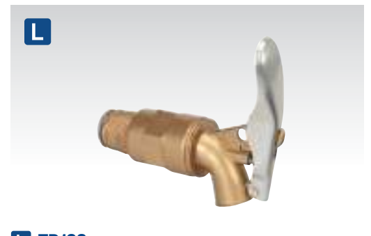
L TP123 3/4" BSP Auto-Release Lockable Drum Tap Self-closing safety drum tap with brass plated alloy body. Features built-in flame arrestor for dispensing flammable or non-flammable liquids. Steel handle can be padlocked closed. Fitted with 3/4" BSP thread.
