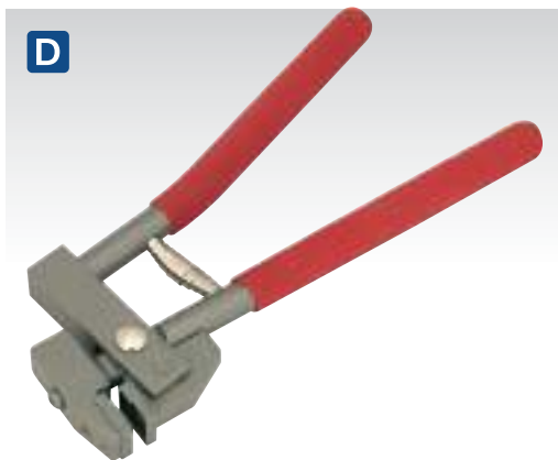
D RE92/30 Joggler/Flanging Tool All steel construction with spring loaded handles. Precision jaws make 10mm flange on 18-20 gauge mild steel or aluminium sheet and provide smooth, flush joint between panels. Fitted with non-slip PVC grips.
