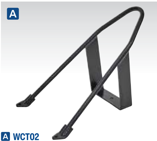
B SEE BELOW Motorcycle Wheel Chocks Black powder coated heavy-duty tubular frame. Pre-drilled holes allow chocks to be bolted to either the floor or a trailer to prevent movement while being worked on or transported.
