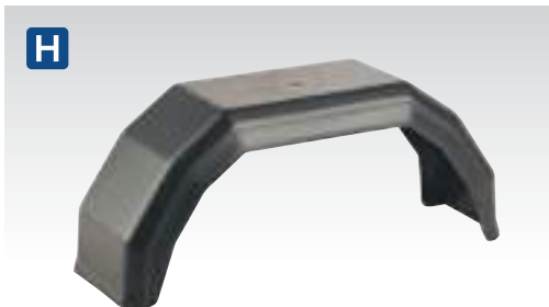
H-J SEE BELOW Mudguards Trailer mudguards, injection moulded in durable high-density polyethylene. H TB31 Mudguard for 200mm(8") Wheels Size (W x D x H): 490 x 140 x 195mm I TB32 Mudguard for 250mm(10") Wheels Size (W x D x H): 620 x 180 x 240mm J TB33 Mudguard for 330mm(13") Wheels Size (W x D x H): 760 x 220 x 335mm
