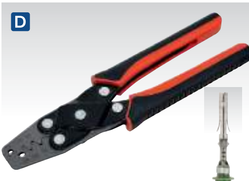
D AK3860 Crimping Tool - Delphi Weather Pack All steel construction with anti-slip handles and hardened and tempered jaws. For use on Delphi Weather Pack terminals. Parallel jaw movement ensures consistent crimp tension. Terminal Suitability: 0.35mm 2 , 0.5-0.8mm 2 , 1-2mm 2 , 3mm 2 Length: 215mm
