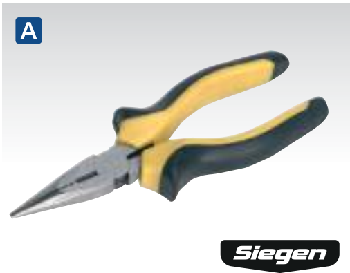
A S0811 150mm Long Nose Pliers Induction heat treated and hardened steel components. Fully chromed and polished jaw head for corrosion resistance. Fitted with oversized grips for extra comfort. Length: 150mm
