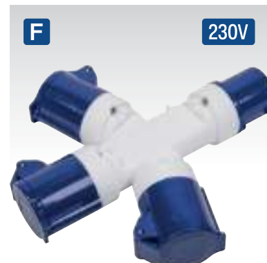
F WTWS16A 3-Way Splitter 230V 3-Way splitter 230V~50Hz, allows splitting of a maximum current of 16A. Fitted with one 2P+E input and three output connectors. IP44 Rated.
