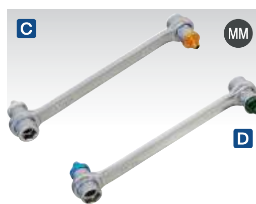
C-D SEE BELOW Double End Brake Bleeder Spanners Specially designed caliper bleed nipple spanners simplify brake bleeding. Fitted with neoprene rubber seals which stops air being put into the system. Colour-coded for easy size identification. Model No: Spanner Sizes: C VS4511 8 x 9mm D VS4512 10 x 11mm
