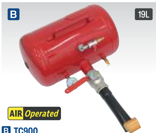
B TC900 19L Bead Seating Tool - Lever Trigger The easy and instant way to seat tubeless tyre beads. Dumps air into tyre void forcing bead to seat against rim for inflation. Air release is controlled by a hand lever operating a ball valve. Fully certified tank with gauge and safety valve prevents over pressurising. Suitable for use on cars, commercials, agricultural and ATV tyres.
