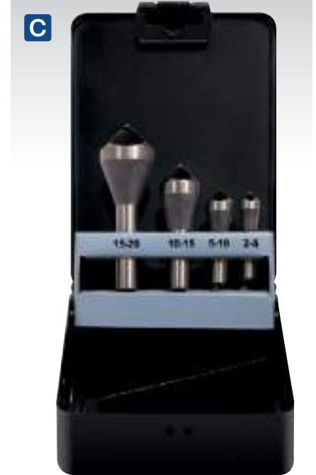
C CSSET40 4pc 90° Slotted Deburring Countersink Drill Bit Set Chip removal through the slot prevents excess waste from clogging the workpiece. Ideal for burr, chatter-free deburring and countersinking. More efficient than a standard countersink. Compatible with wood and light metals. Supplied in a metal storage case. Contents: Ø2-5, 5-10, 10-15, 15-20mm
