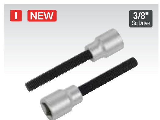
I VS0572 2pc 3/8" Sq Drive Brake Drum Remover Designed to thread into the brake drums M8 x 1.25mm access points. Removes stuck brake drums safely and efficiently. To be used as a pair so that the drum is removed smoothly and squarely. 3/8" Sq drive.
