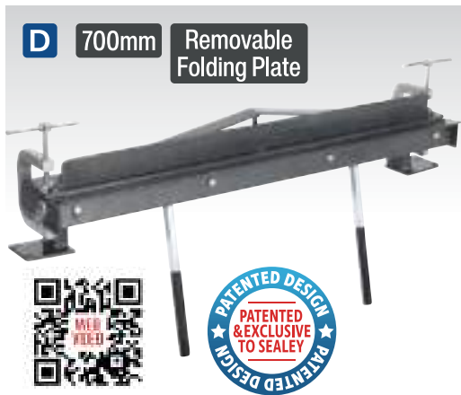
D TS01 700mm Vice/Bench Mounting Sheet Metal Folder Bench and vice mounting sheet metal folder, fitted with mounting plates. Capable of bending up to and beyond a 90° angle. The unique patented 'endless' design and removable folding plate allows the user to fold, channel and offset any length of sheet metal up to 20 Gauge/0.91mm thick. Capable of two folds at right angles to each other to form a corner piece. With adjustable fold plate to help achieve the cleanest fold possible. Ideal for the small garage or restoration operation. Capacity: 700mm x 20 Gauge Sheet, Ø1mm Rod
