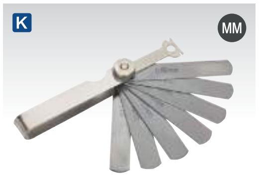
K VS518 Spark Plug Feeler Gauge Specially designed for gapping spark plugs and suitable for both traditional copper and precious metal plugs. Features an electrode adjuster allowing the electrode to be adjusted without levering against the core which can be easily damaged. Blade dimensions 75 x 13mm. Blade Sizes: 0.5, 0.6, 0.7, 0.8, 0.9, 1, 1.1mm
