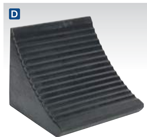
D WC12 Heavy-Duty Rubber Wheel Chock 12kg - Single Heavy-duty nylon reinforced rubber wheel chock. Prevents vehicle movement when being jacked on a level surface or parked on an incline not exceeding 12°. Features robust carry handle that can also be fitted with a rope or chain (not included). Suitable for commercial, agricultural and aircraft tyres of Ø1500-1800mm. Suitable for vehicles below 40 Tonne. Dimensions (W x D x H): 300 x 255 x 300mm
