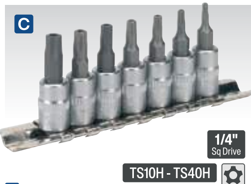
C SX106 7pc 1/4" Sq Drive TRX-TS* Security Socket Bit Set Chrome Vanadium steel sockets and bits. Knurled ring on sockets to assist gripping with oily fingers. 5-Spline security TRX-TS* bits suitable for a range of fuel injection applications. Supplied on socket rail. Drive: 1/4" Sq Contents: TS10H, TS15H, TS20H, TS25H, TS27H, TS30H, TS40H
