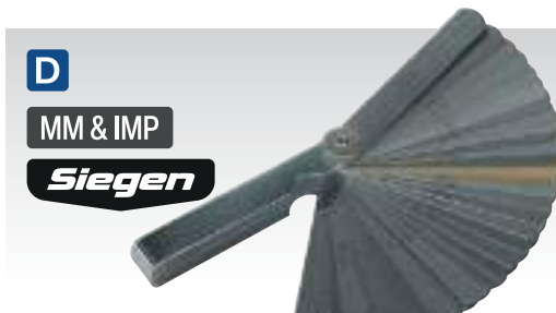
D S0514 32 Blade Feeler Gauge - Dual Marked Includes 0.010" (0.254mm) brass blade for non-magnetic applications. Blade dimensions 90 x 13mm. Blade Sizes: Imperial: 0.0015", 0.002", 0.0025", 0.003", 0.004", 0.005", 0.006", 0.007", 0.008", 0.009", 0.010", 0.011", 0.012", 0.013", 0.014", 0.015", 0.016", 0.017", 0.018", 0.019", 0.020", 0.021", 0.022", 0.023", 0.024", 0.025", 0.026", 0.028", 0.030", 0.032", 0.035" + 0.010" Brass Metric: 0.038, 0.051, 0.063, 0.076, 0.102, 0.127, 0.152, 0.178, 0.203, 0.229, 0.254, 0.279, 0.305, 0.330, 0.356, 0.381, 0.406, 0.432, 0.457, 0.483, 0.508, 0.553, 0.559, 0.584, 0.610, 0.635, 0.660, 0.771, 0.762, 0.813, 0.889 + 0.254mm Brass
