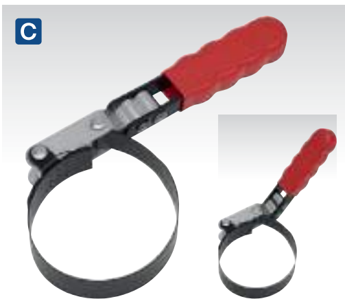
C MS046 Ø60-84mm Oil Filter Band Wrench Suitable for removing and installing oil filters with diameters ranging from Ø60-84mm. 25mm Wide spring steel band with corrosion resistant coating. PVC dipped multi-position handle can be applied at 180° to the filter. Automatically tightens as pressure is applied.
