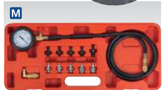
M VSE203 12pc Oil Pressure Test Kit Ø65mm Gauge fitted with heavy-duty cover. Tests oil pump pressure and also low oil warning devices. Fitted with quick coupling adaptors and 1.3m hose. Includes 90° coupling adaptor for limited access applications. Adaptors: 1/8" DIN 2999, 1/8" x 27NPT, 1/4" x 18NPT, 3/8" x 20UNF, 1/2" x 20UNF, M10 x 1, M12 x 1.5, M14 x 1.5, M16 x 1.5, M18 x 1.5mm, 90° Elbow
