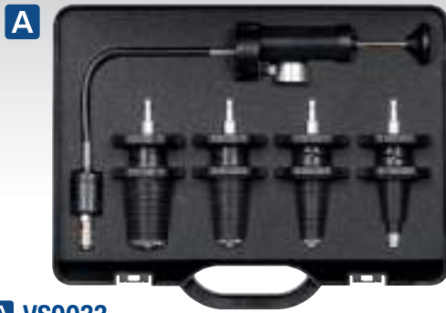
A VS0033 5pc Cooling System Pressure Test Kit Capless tester uses cone adaptor system to seal and pressurise the cooling system. Adaptors may be used to replace both screw and bayonet type cap fittings. Kit includes pump with gauge and four system adaptors for use on a wide range of vehicle applications. Contents: Cone Adaptor Sizes; 17-24, 28-31.5, 37-39.5, 47-48.5mm
