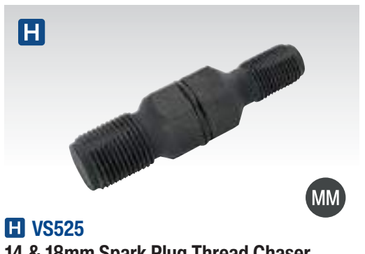
H VS525 14 & 18mm Spark Plug Thread Chaser Suitable for cleaning corrosion and carbon build-up from spark plug threads. Also possible to restore minor cross threading damage. Use with a 21mm spark plug socket. Size: 14, 18mm Thread Lengths: 14-15mm, 18mm Maximum Drive Diameter: Ø21mm
