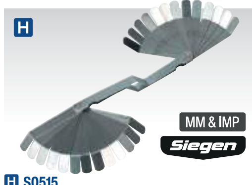
H S0515 26 Blade Offset Feeler Gauge - Dual Marked Offset tips are essential for checking tolerances on OHC configurations and suitable for other applications where straight blades will not fit. Blade dimensions 100 x 12.7mm (45°-25mm offset). Blade Sizes: Imperial: 0.005", 0.006", 0.007", 0.008", 0.009", 0.010", 0.011", 0.012", 0.013", 0.014", 0.015", 0.016", 0.017", 0.018", 0.019", 0.020", 0.021", 0.022", 0.023", 0.024", 0.025", 0.026", 0.027", 0.028", 0.029", 0.030" Metric: 0.127, 0.152, 0.178, 0.203, 0.229, 0.254, 0.279, 0.305, 0.330, 0.356, 0.381, 0.406, 0.432, 0.457, 0.483, 0.508, 0.533, 0.559, 0.584, 0.610, 0.635, 0.660, 0.686, 0.711, 0.737, 0.762mm
