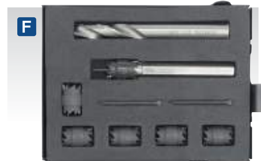
F AK4730 9pc Ø10mm Spot Weld Cutter & Drill Bit Set Suitable for drilling out spot welds on most vehicle panels. Spot weld cutter features spring loaded centre point to guide cutting crown onto weld. Ø8mm HSS Drill with 5% Cobalt for longer life, suitable for more specialist materials including galvanized, boron and high stress steels. Solid Cobalt stock allows resharping, extending product life. Set includes replacement centre points and cutter crowns. Supplied in metal storage case. Contents: Spot Weld Cutter, Ø8mm Cobalt Spot Weld Drill, Centre Points (x2), Ø10mm Cutter Crowns (x5) Spot Weld Cutting Crown (Pack of 2): Z1C2
