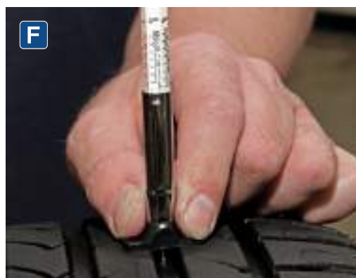
F TST/DGE Tyre Tread Depth Gauge - Pocket Type Chromed steel body with pocket-clip. Scale from 0-25mm in 1mm(0-1" in 1/32") graduations.
