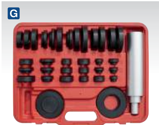
G VS7024 37pc Bearing & Seal Installation Kit Lightweight design for the installation of bearings without damaging the bearing or housing. Contains three metal bearing drift sleeves and 34 nylon drifts. Can also be used to install oil seals. Fits most sizes of bearing and seals found on modern vehicles. Supplied in storage case.
