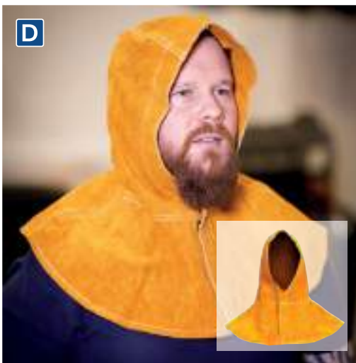
D SSP145 Heavy-Duty Leather Welding Safety Hood Heavy-duty leather welding hood, offers best mix of durability, comfort and protection from sparks and spatter. Hook-and-loop fastening means one size fits all. Manufactured from split cow hide leather with Kevlar® stitching. Conforms to EN ISO 11611.
