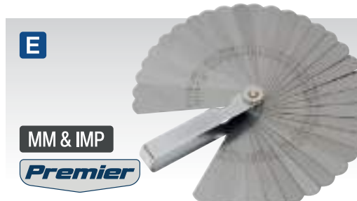
E VS512 35 Blade Feeler Gauge - Dual Marked Blade dimensions 75 x 13mm. Blade Sizes: Imperial: 0.0015", 0.002", 0.003", 0.004", 0.005", 0.006", 0.007", 0.008", 0.009", 0.010", 0.011", 0.012", 0.013", 0.014", 0.015", 0.016", 0.017", 0.018", 0.019", 0.020", 0.021", 0.022", 0.023", 0.024", 0.025", 0.026", 0.027", 0.028", 0.029", 0.030", 0.031", 0.032", 0.033", 0.034", 0.035" Metric: 0.038, 0.051, 0.076, 0.102, 0.127, 0.152, 0.178, 0.203, 0.229, 0.254, 0.279, 0.305, 0.330, 0.356, 0.381, 0.406, 0.432, 0.457, 0.483, 0.508, 0.533, 0.559, 0.584, 0.610, 0.635, 0.660, 0.686, 0.711, 0.737, 0.762, 0.787, 0.813, 0.838, 0.864, 0.889mm
