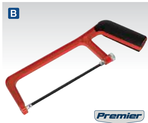
B AK8680 150mm Junior Hacksaw with Adjustable Blade Rigid die-cast aluminium frame with comfortable composite handle. Multi-position clamp permits blade to be mounted at different angles. Supplied with 150mm general-purpose blade. Replacement Blades (Pack of 10): S0527.B
