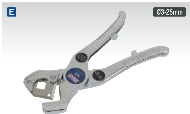
E HCA25 Rubber & Reinforced Hose Cutter Die-Cast Alloy Die-cast zinc alloy body with simple plier action. Suitable for hoses from Ø3-25mm. Simple reversible steel blade hardened and tempered to 50-55 HRC. Supplied in pouch. Capacity: Ø3-25mm Length: 190mm Replacement Blade: HCA25/B
