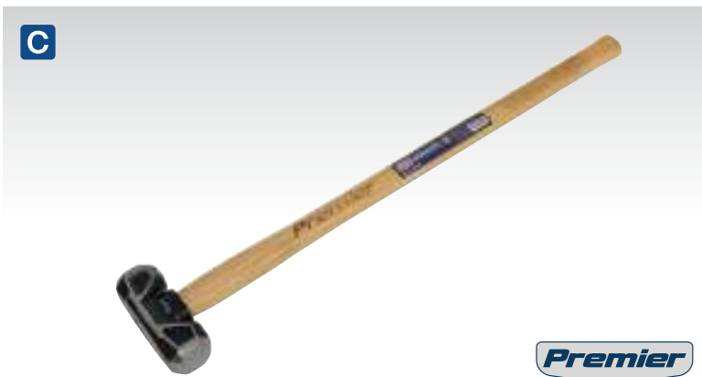
C SEE BELOW Sledge Hammers with Hickory Shaft Manufactured from drop-forged fine grained carbon steel. Heat treated, hardened and tempered with precision ground polished striking face. Straight-grain hickory handle. Manufactured and tested to BS 876.
