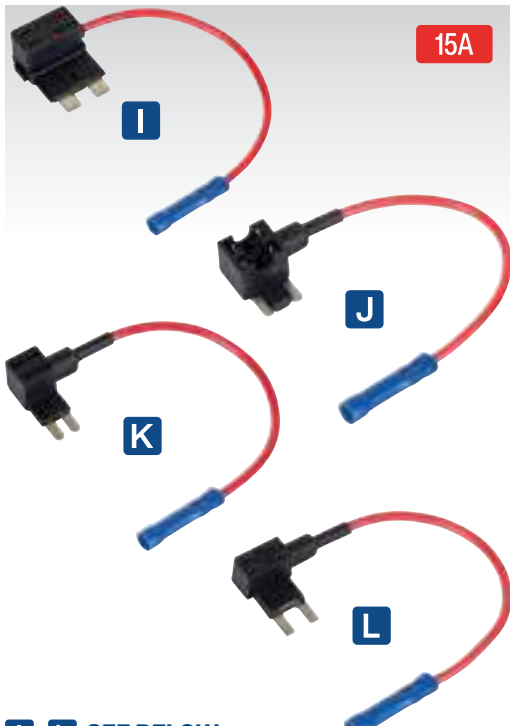
I-L SEE BELOW 15A Accessory Circuit Fuse Holder Links Packs of 2 Range of fuse holders for quick and easy installation of an accessory circuit. Simply remove an existing fuse and insert the fuse holder. Contains two fuse slots, one for the vehicles existing fuse and a second fuse slot for the accessory. Made from nylon and supplied with 150mm of 16 gauge wire. Maximum rated current 15A.
