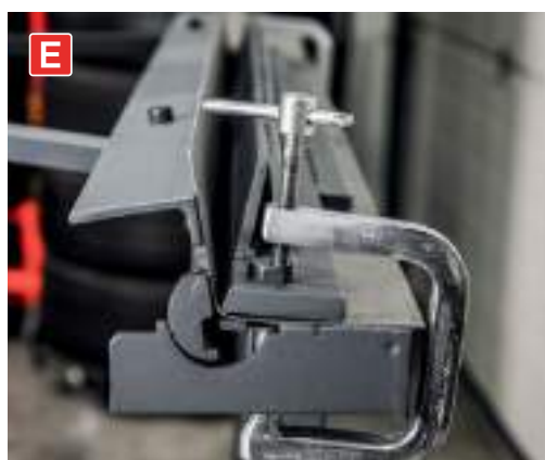
D-E Patented 'endless' design enables shaping of unlimited lengths of metal.
