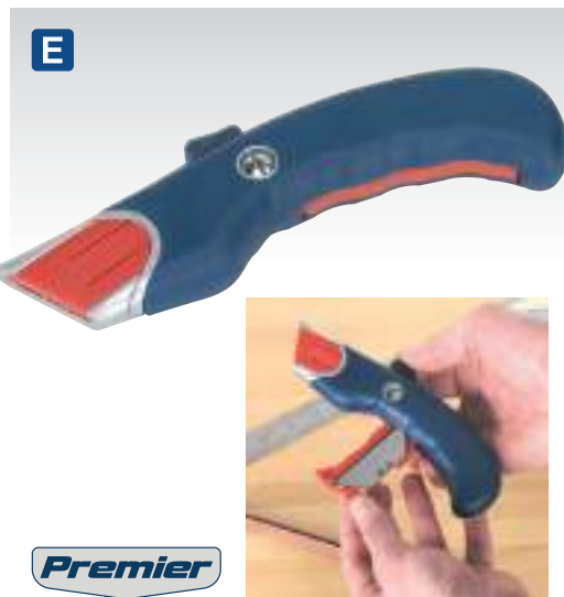
E AK8631 Auto-Retracting Safety Knife Ergonomically profiled zinc alloy body with comfort grip. Features auto-retracting blade which prevents inadvertent exposure of cutting edge and subsequent injury/damage. Satisfies HSE requirements. Push-release cover for quick blade removal/fitting - no tools required. Integral blade storage in body of knife with push-button release.
