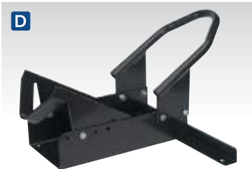
D FPS4 Motorcycle Rear Wheel Chock Features adjustable pivoting wheel guide, which secures rear wheel within chock. Four adjustable depths depending on diameter of wheel. Suitable for wheels with tyre widths Ø130-180mm and diameters Ø14"-21" (Ø355-535mm). Frame bolts to the floor, stabilising motorcycles without the need of side or centre-stands. Min./Max. Tyre Width: 130-180mm Min./Max. Wheel Diameter: Ø14"-21" (Ø355-535mm)
