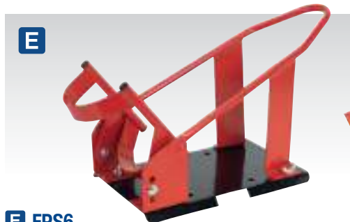
E FPS6 Motorcycle Front Wheel Chock Features adjustable pivoting wheel guide, which secures front wheel within chock. Three adjustable heights depending on diameter of wheel. Suitable for wheels with tyre widths 90-130mm and diameters Ø17"-21" (Ø430-535mm). Base can be permanently bolted to the floor (fixings included), and features a detachable upper assembly that can be easily stored and re-attached when required, stabilising motorcycles without the need for side or centre-stands. Base features lashing strap gap for securing the bike in transport. Min./Max. Tyre Width: 90-130mm Min./Max. Wheel Diameter: Ø17"-21" (Ø430-535mm)
