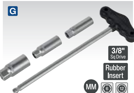
G AK6550 4pc 3/8" Sq Drive T-Bar & Rubber Insert Spark Plug Socket Set Comfort grip T-handle 3/8" Sq drive. Features 2-in-1 wobble and rigid bar. Simply push the socket further onto the bar to fasten in the rigid position. Includes 14mm Bi-hex, 16 and 21mm 6-point Chrome Vanadium spark plug sockets with rubber inserts. Drive: 3/8" Sq Sizes: 14, 16, 21mm
