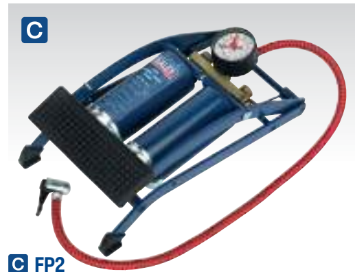
C FP2 Twin Barrel Foot Pump High power, steel framed foot pump with two Ø50 x 120mm steel barrels. Dial type pressure gauge with rotating bezel. Gauge calibrated in psi and bar and ranges from 0-100psi and 0-7bar. Fitted with 610mm flexible pressure hose with locking connector.
