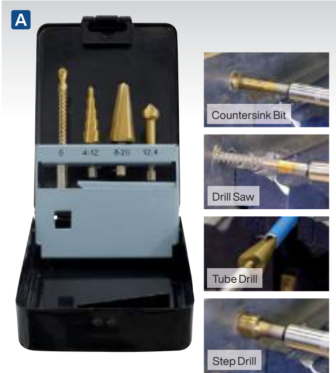
A AK4704 4pc Multifunction Drill Bit Set Multifunction drill bit set to cover most of your drilling needs. Set includes a drill saw, step drill, tube drill and countersink. Drill saw bit can be used as a drill, saw, rotary file, reamer and router. Contents: Ø4-12mm Step Drill, Ø8-20mm Tube Drill, Ø6mm Drill Saw, Ø12.4mm Countersink
