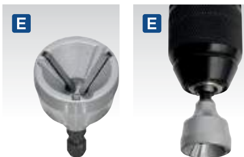
E DB04 Ø3-19mm External Deburring/Chamfer Tool Designed to clean up and repair threaded fasteners and studding quickly and safely. Fitted with 3 x HSS blades to remove damaged metal and burrs. Features a 1/4" Hex shank for use with a drill or hex driver. Applicable for use on pieces from Ø3mm to 19mm in diameter. Suitable for use with a variety of compounds including stainless steel, hardened steel, mild steel, copper, brass, plastic and many more. Unit is much faster and more accurate than using a file or angle grinder. Applications: Stainless Steel, Hardened Steel, Mild Steel, Copper, Brass, Wood, Plastic, Fibreglass
