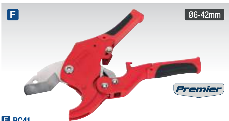
F PC41 Plastic Pipe Cutter Powder coated aluminium body. Operates with a simple plier action. Ratchet cutting action and quick release mechanism. Heat treated stainless steel cutting blade. Fitted with safety lock and comfort grip handles. Suitable for plastic pipe from Ø6-42mm. Capacity: Ø6-42mm Length: 210mm
