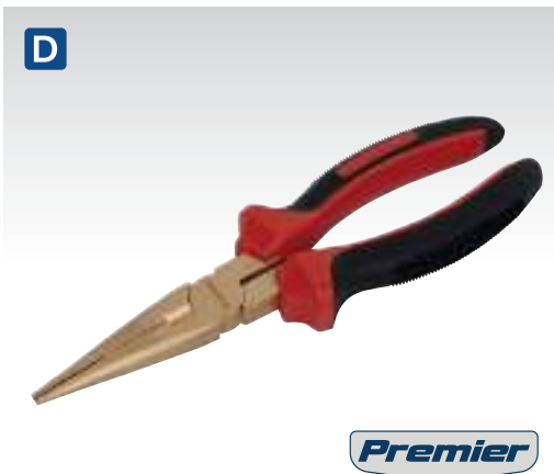
D NS075 200mm Long Nose Pliers - Non-Sparking Manufactured from Beryllium Copper. Die Forged. Serrated jaw and hardened cutters. Dual material handle for greater comfort and control.
