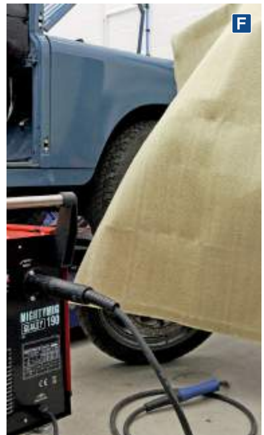
F SSP233 Fibreglass Spark Proof Welding Blanket Glass fibre blanket treated with a mineral based aqueous dispersion. Will withstand temperatures of up to 1000°C. Protects against the spray of sparks from welding and cutting applications.
