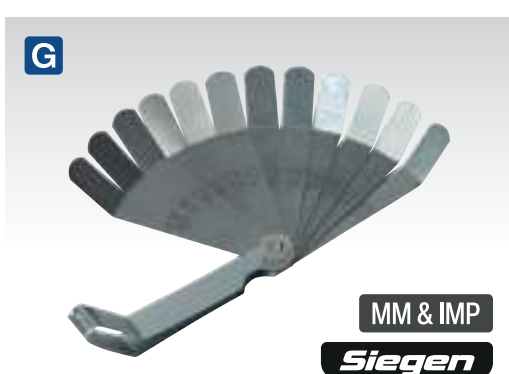
D S0514 32 Blade Feeler Gauge - Dual Marked Includes 0.010" (0.254mm) brass blade for non-magnetic applications. Blade dimensions 90 x 13mm. Blade Sizes: Imperial: 0.0015", 0.002", 0.0025", 0.003", 0.004", 0.005", 0.006", 0.007", 0.008", 0.009", 0.010", 0.011", 0.012", 0.013", 0.014", 0.015", 0.016", 0.017", 0.018", 0.019", 0.020", 0.021", 0.022", 0.023", 0.024", 0.025", 0.026", 0.028", 0.030", 0.032", 0.035" + 0.010" Brass Metric: 0.038, 0.051, 0.063, 0.076, 0.102, 0.127, 0.152, 0.178, 0.203, 0.229, 0.254, 0.279, 0.305, 0.330, 0.356, 0.381, 0.406, 0.432, 0.457, 0.483, 0.508, 0.553, 0.559, 0.584, 0.610, 0.635, 0.660, 0.771, 0.762, 0.813, 0.889 + 0.254mm Brass
