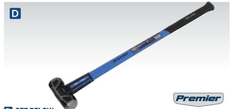
D SEE BELOW Sledge Hammers - Fibreglass Shaft with Graphite Core Manufactured from drop-forged fine grained carbon steel. Heat treated, hardened and tempered with precision ground polished striking face. Domed strike zone for power and efficiency. Fibreglass shafts with graphite core for improved strength and durability. Textured rubber grip for secure handling. Manufactured and tested to BS 876.
