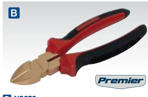
B NS073 200mm Diagonal Cutting Pliers - Non-Sparking Manufactured from Beryllium Copper. Die forged diagonal cutters. Hardened cutting jaws with dual material grip for improved comfort and control.
