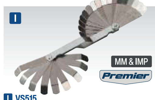
I VS515 26 Blade Offset Feeler Gauge - Dual Marked Offset tips are essential for checking tolerances on OHC configurations and suitable for other applications where straight blades cannot reach. Blade dimensions 75 x 13mm (45°-15mm offset). Blade Sizes: Imperial: 0.005", 0.006", 0.007", 0.008", 0.009", 0.010", 0.011", 0.012", 0.013", 0.014", 0.015", 0.016", 0.017", 0.018", 0.019", 0.020", 0.021", 0.022", 0.023", 0.024", 0.025", 0.026", 0.027", 0.028", 0.029", 0.030" Metric: 0.127, 0.152, 0.178, 0.203, 0.229, 0.254, 0.279, 0.305, 0.330, 0.356, 0.381, 0.406, 0.432, 0.457, 0.483, 0.508, 0.533, 0.559, 0.584, 0.610, 0.635, 0.660, 0.686, 0.711, 0.737, 0.762mm
