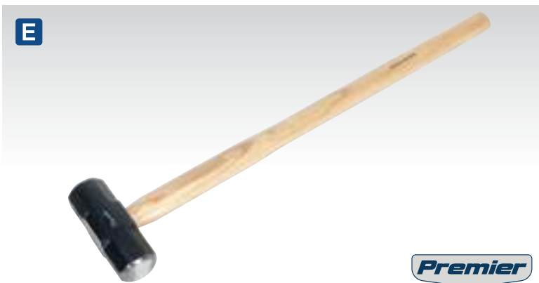
E SEE BELOW Sledge Hammers with Hickory Shaft Manufactured from fine grained alloy steel, heat treated, induction-hardened and tempered with double precision ground polished striking face. Fitted with straight-grained hickory shaft. Manufactured in accordance with BS 876.
