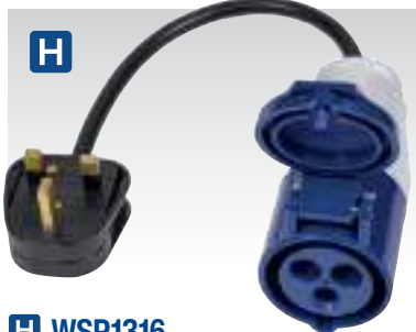
H WSP1316 13A/16A Trailing Socket & Cable Set Trailing socket and cable fitted with a 230V~50Hz 13A standard UK plug and 2P+E socket rated at 230V~50Hz 16A. H05VV-F 3G 1.5mm Section cable, 350mm in length. IP20 Rated. Length: 350mm Cable
