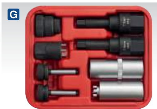
G VS2068 8pc Diesel Injector Repair Socket Set Suitable for repairs on Bosch, Denso and Siemens injectors. 6.6, 7.6mm Hex security bits 20mm Hex/1/2" Sq Drive. 16mm 8-sided socket for Bosch common rail Injectors. Denso common rail injector valve seat removal tool. Injector ball valve lapping tools and guide. Manufactured from Chrome Vanadium steel and S45C. Supplied in storage case. Drive: 1/2" Sq Applications: Bosch, Denso and Siemens injectors
