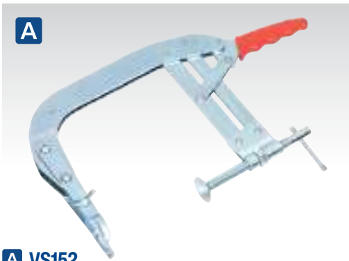
A VS152 OHV Valve Spring Compressor Suitable for most small and medium sized OHV engines. Fully adjustable jaw with 75-165mm capacity and 150mm throat depth. Parallel lift action with automatic lock.
