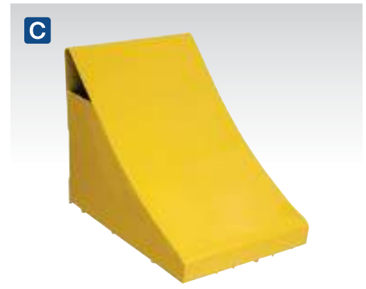
C WC18 Heavy-Duty Steel Wheel Chock - Single Welded steel wheel chock. Prevents vehicle movement when being jacked on a level surface or parked on an incline not exceeding 10°. Suitable for heavy goods vehicles not exceeding 20 Tonne gross weight.
