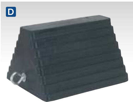
D WC03 Rubber Wheel Chock 3.8kg - Single Single nylon reinforced rubber wheel chock. Prevents vehicle movement when being jacked on a level surface or parked on an incline not exceeding 12°. Fitted with eye bolt for rope or chain. Suitable for vehicles below 10 Tonne.
