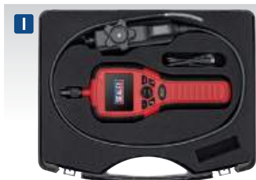
I VS8233A Ø6mm Video Borescope - Articulated Portable articulated borescope supplied with 70mm TFT colour display. Mini waterproof (IP67) camera with integral light (Ø6mm) mounted on 800mm flexible 2-way articulated probe. Using an attached dial, the camera head angle can be changed by up to 350° without having to remove camera from inspection area. Using 8GB micro SD card (supplied) up to 9hrs of video and 20000 still images can be recorded. Videos and still images can be downloaded to a PC via USB data cable (supplied). CMOS camera with six LED probe light and a focus distance of 20-50mm for fine control of light output and clear pictures. Potential applications; automobile maintenance, engine inspection, pipe line exploration etc. Powered by 4 x AA batteries (not included). Camera Probe Length: 800mm Camera: Ø6mm Mirror Flip/Rotate Function: ✓ Pod Length: 20mm Power Source: 4 x AA Batteries (not included)
