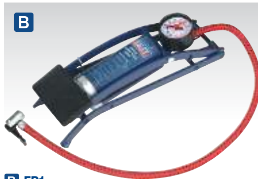
B FP1 Single Barrel Foot Pump Steel framed foot pump with Ø50 x 120mm steel barrel. Dial type pressure gauge with rotating bezel. Gauge calibrated in psi and bar and ranges from 0-100psi and 0-7bar. Fitted with 610mm flexible pressure hose with locking connector. Supplied with accessory for inflating items such as small inflatable boats, air beds and balls.
