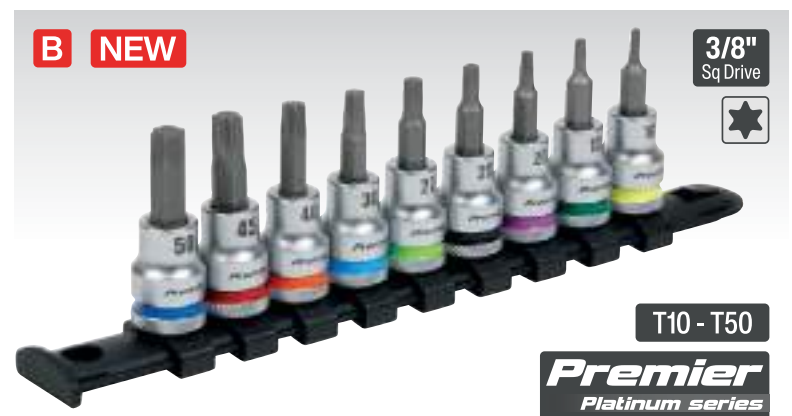
B AK6251 9pc 3/8" Sq Drive TRX-Star* Socket Bit Set - Platinum Series Forged Chrome Vanadium steel sockets with S2 steel TRX-Star* bits. Sockets are heat treated and chrome plated with a fully polished micro satin finish. Colour-coded rings for fast identification. Knurled rings assist the gripping of the sockets with oily fingers. Drive: 3/8" Sq Contents: T10, T15, T20, T25, T27, T30, T40, T45, T50
