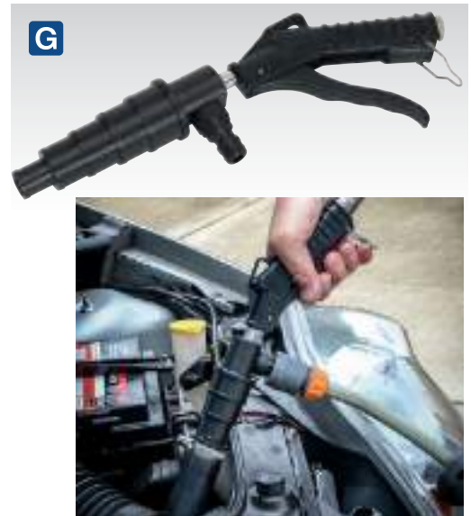
G VS0044 Coolant System Flush Gun Enables thorough flushing of debris and contaminants from cooling system during repair and maintenance. Powered by workshop air, which creates a vacuum to draw water from a container. Can also be used with mains pressure tap water. Adaptor Sizes: Ø19, Ø29, Ø32, Ø37, Ø40mm Air Inlet Size: 1/4" BSP Water Inlet Size: Ø15.5mm Operating Pressure: 90psi
