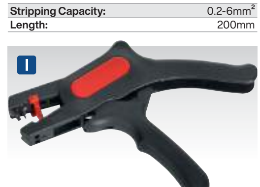
I AK2265 Automatic Pistol Grip Wire Stripping Tool Automatic wire stripper and cutter operates in one easy single-handed operation. Features a handle lock and adjustable wire stop. Manufactured from reinforced fibreglass and nylon with hardened steel blades. Stripping Capacity: 0.2-6mm 2 Maximum Cutting Capacity: 2mm 2 Maximum Stripping Length: 12mm
